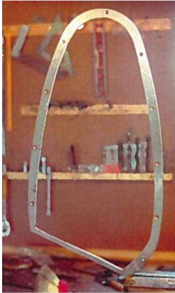
A Duralumin Spacer-plate, to carry out the Chaincase cover to make room for the Chunky Racing Clutch
