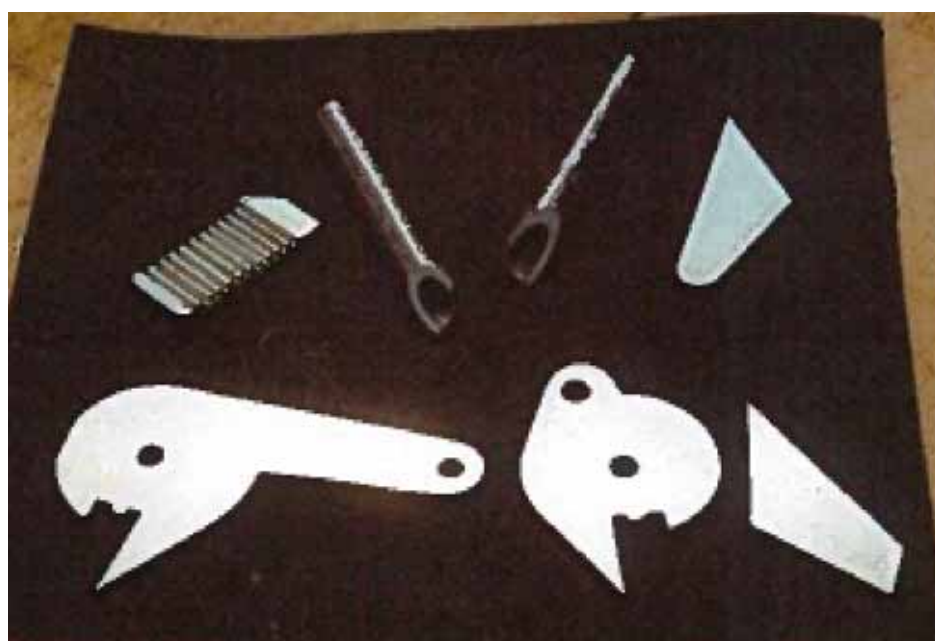
Mild steel, hand-cut parts, highly polished, ready for welding together & then chroming
